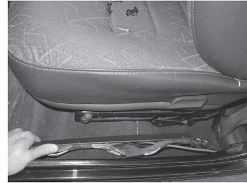
**6.** Use a Phillips screw driver to remove the three clips holding the factory wire harness under the door threshold on the drivers' side.
