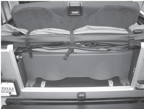
4. If externally amplified, make speaker connections to the enclosure from the amplifier. Connect speaker wires from amplifier to enclosure, positive to red terminal and negative to black terminal.
